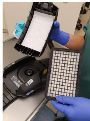
**Photo 6.** Filters in airpump.
