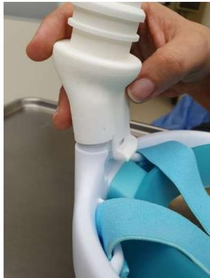
**Photo 3.** 3D-printed connector between hose and mask.
